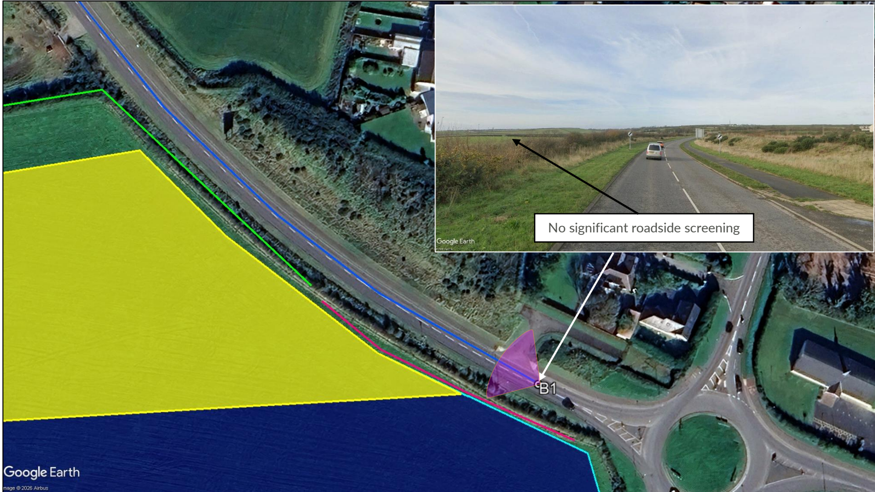
Figure 13 Reflective panel area and proposed screening for road receptor B1
