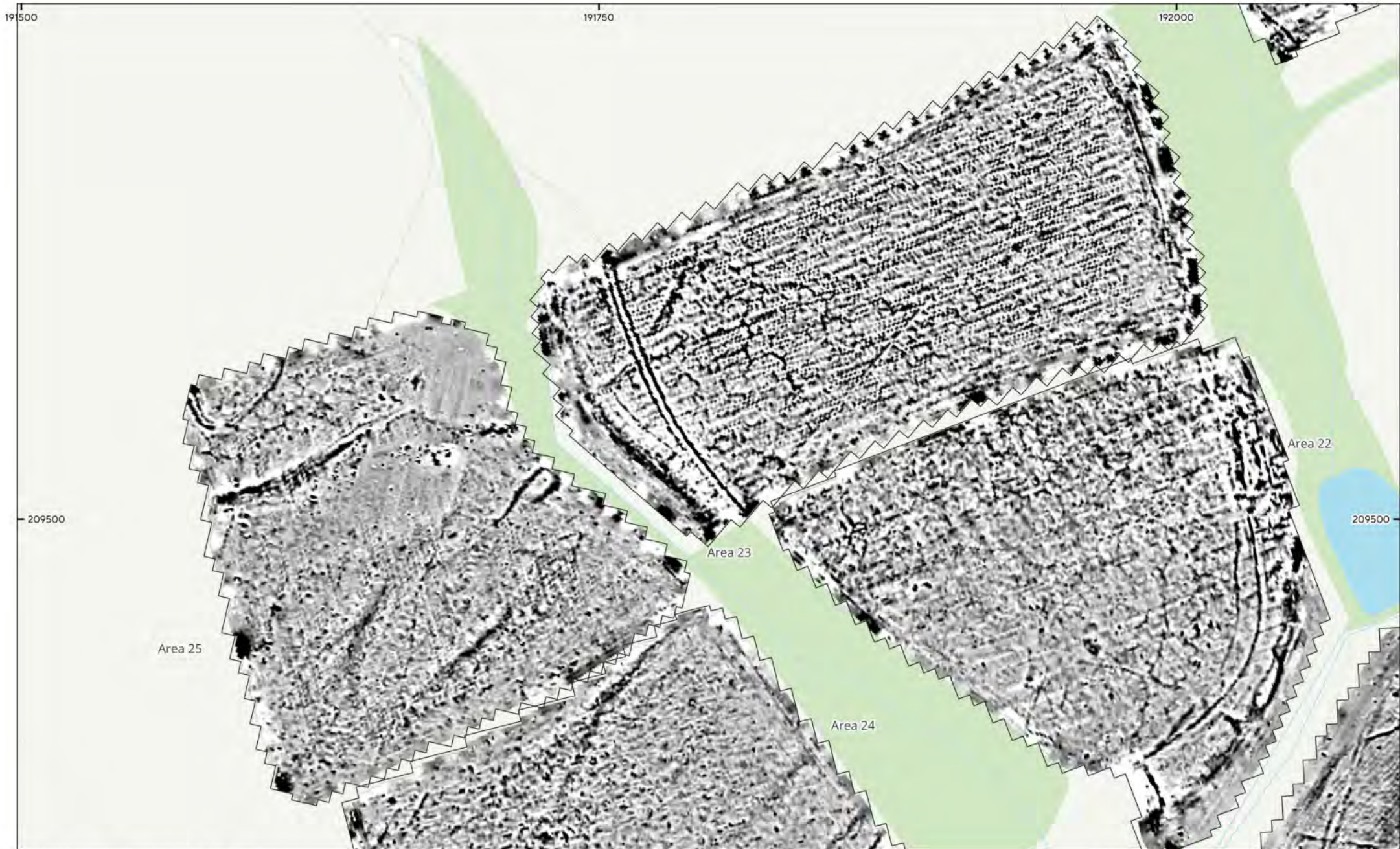
MSSM2260 - Great Harmeston Solar Farm Figure 30 - Magnetic Gradient (Areas 22, 23, 24 (North) & 25) 1:1,500 @ A3 © Magnitude Surveys 2026 Contains Ordnance Survey data © Crown Copyright and database right 2026
