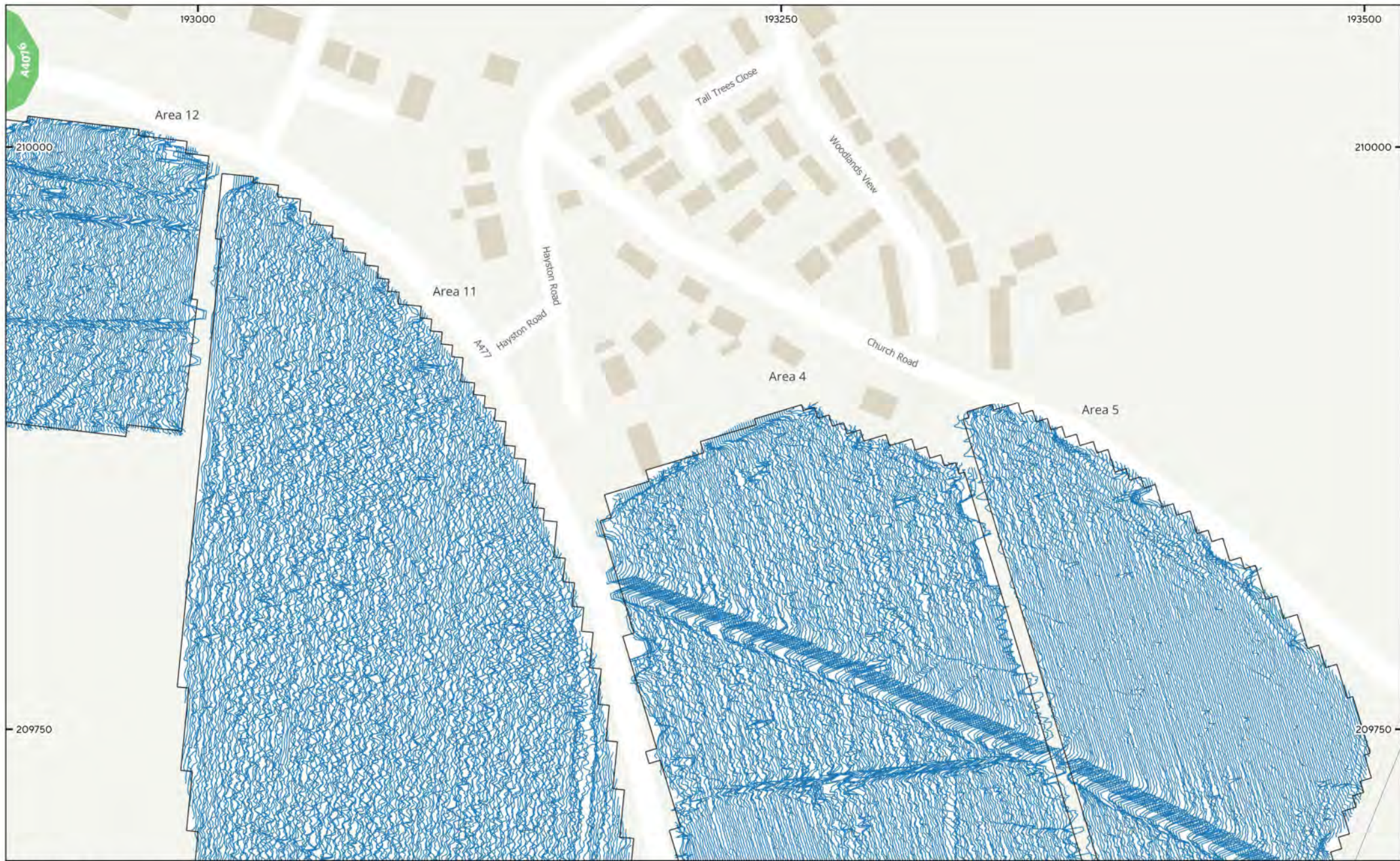
MSSM2260 - Great Harmeston Solar Farm Figure 26 - XY Plot (Areas 4 (North), 5 (North), 11 (North) & 12 (East)) 1:1,500 @ A3 90nT/cm at 1:1,500 @ A3 © Magnitude Surveys 2026 Contains Ordnance Survey data © Crown Copyright and database right 2026
