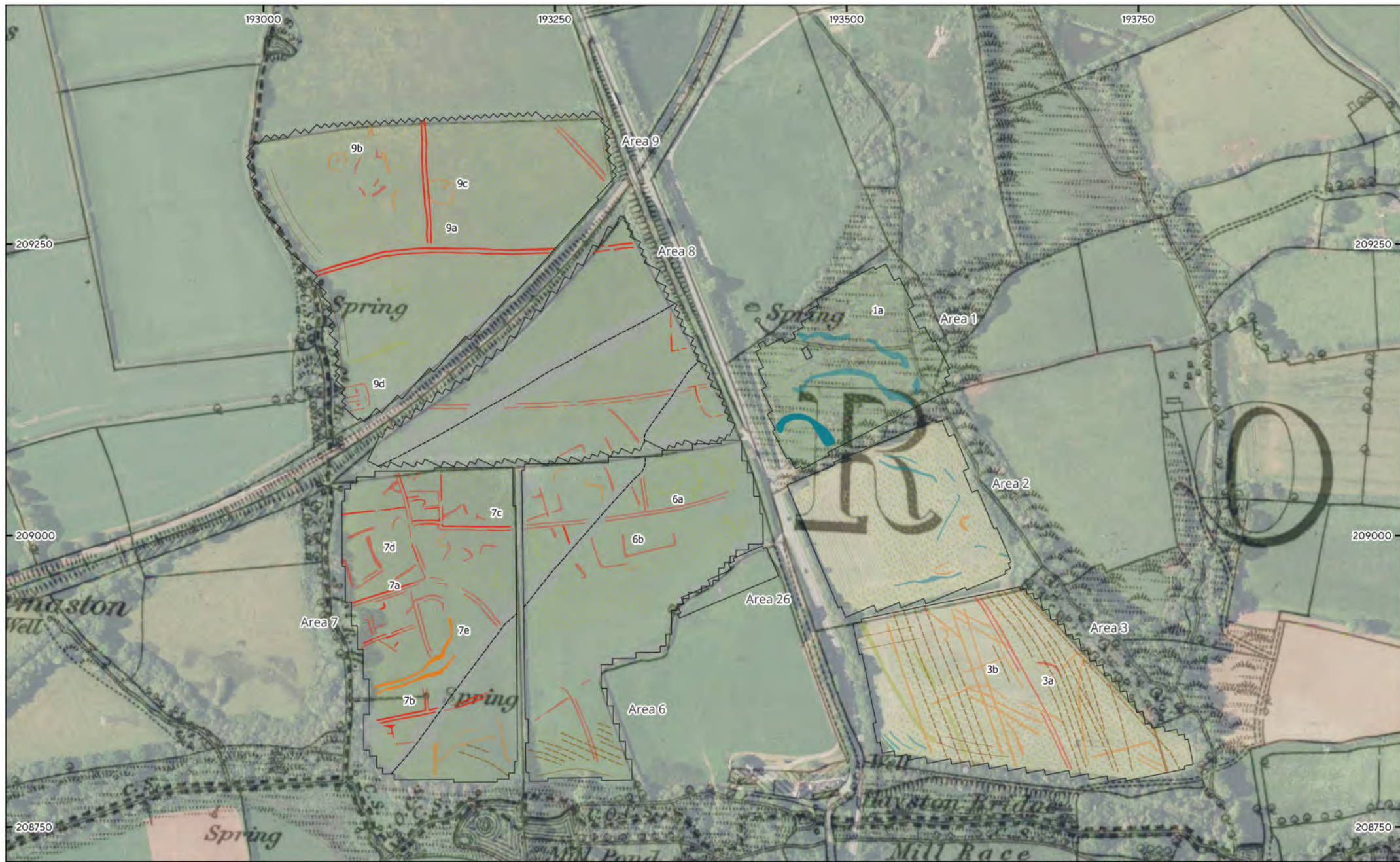
MSSM2260 - Great Harmeston Solar Farm Figure 13 - Magnetic Interpretation over Historical Mapping and Satellite Imagery Overview (Areas 1-3, 7-9 & 26) 1:3,000 @ A3 © Magnitude Surveys 2026 Contains Ordnance Survey data © Crown Copyright and database right 2026
