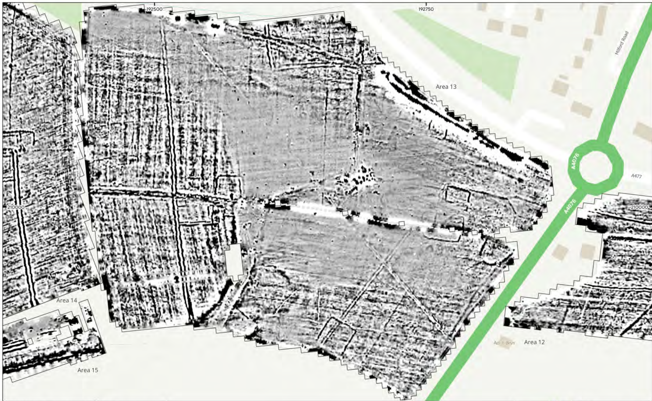
MSSM2260 - Great Harmeston Solar Farm Figure 21 - Magnetic Gradient (Areas 12 (West), 13, 14 (East) & 15 (East)) 1:1,500 @ A3 © Magnitude Surveys 2026 Contains Ordnance Survey data © Crown Copyright and database right 2026
